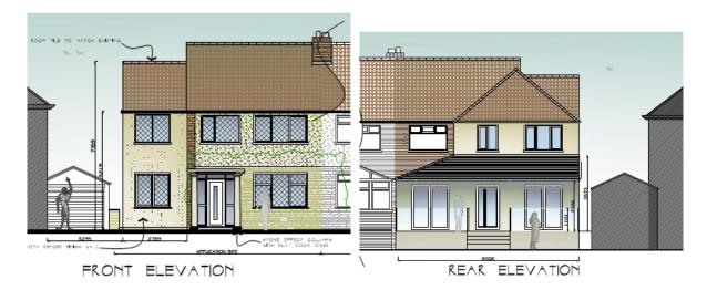
The rear first floor extension projects 4.3m and is set back 3m from the boundary to protect the 45 degree rule of thumb.
